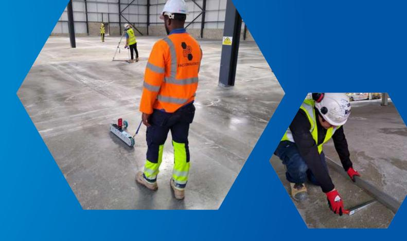
**Relative Humidity Testing** - checks whether the moisture level of the concrete has reduced to a value where resilient flooring can be safely laid.
